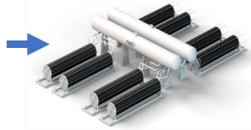
Hydrogen Production facility – Electrolysers, compressors and supporting infrastructure
