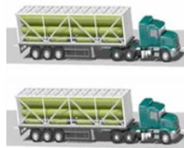
Specialised tube trailer for storage and distribution
